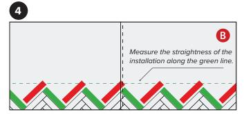
Now install **B-strips** and cut the most right piece to size.
