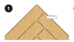
Measure the distance between the two straight lines, originating from the corners of the strips.
