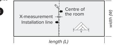
**Drawing the installation line.**Start from the center of the room.
