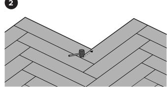
Use a rubber hammer and slightly knock at the 5Gi system to connect the short side. Start in the corner and work towards the end of the board.
