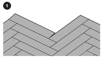
The boards need to be locked into one another, using the 5Gi system. To connect a new board you have to use a rubber hammer.
