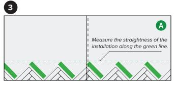
Install **A-strips** to connect all triangles. The joints between the A-strip and the triangle need to be checked very carefully. No protruding edge may be felt! Cut the most left piece to fit into the room, concidering an expansion gap.
