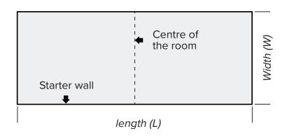
Define the wall from where you intend to start the installation. Mark out the center of the room.
