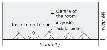
Lay out the triangles with their long side towards the starting wall. Align the center triangle top with the installation line.
